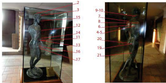
Figure 5: P-EDXRF analysis places from different points of sculpture
